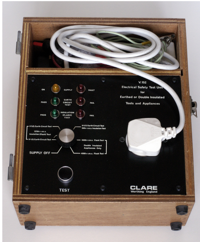
Figure 5.1 Older PAT testers are still perfectly capable of safety testing.
