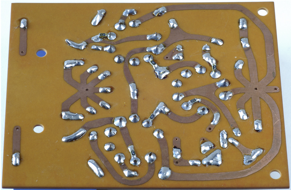
Figure 3.46 Star earth and power on a PCB.
