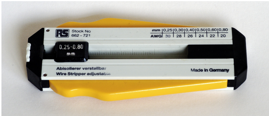
Figure 3.9 Calibrated stripper for fine wires.
