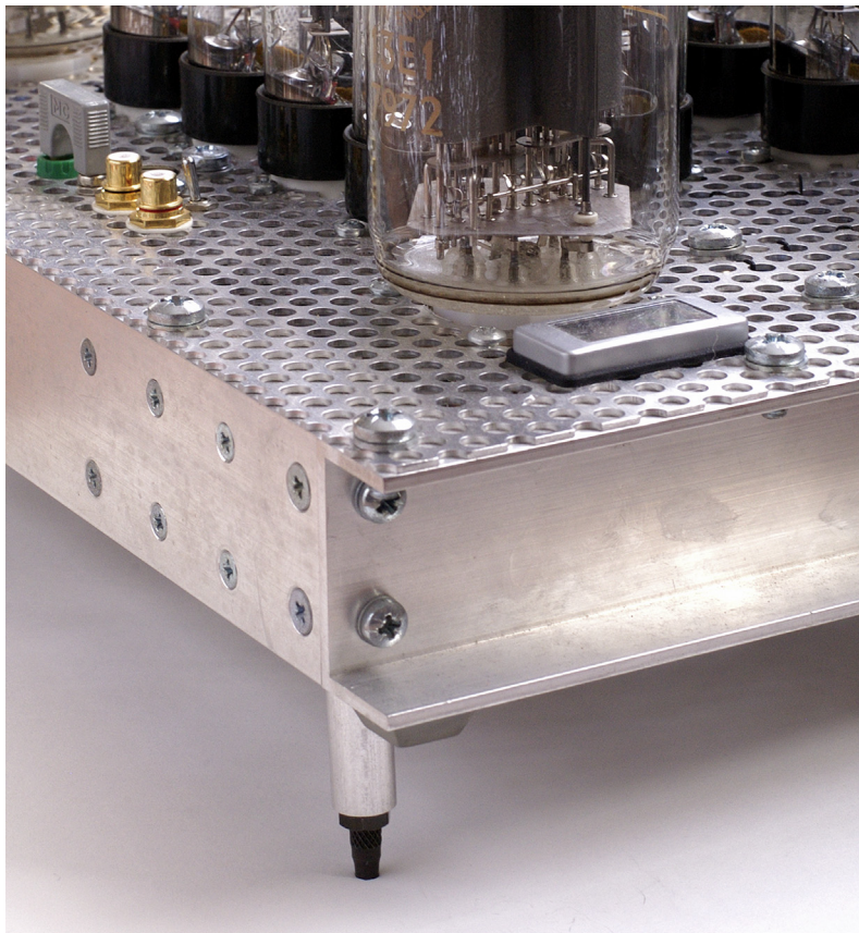
Figure 1.11 Perforated sheet and tall feet allow excellent cooling.
