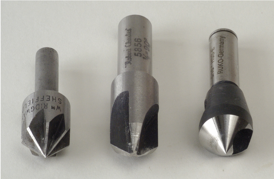
Figure 2.19 Selection of countersinks.
