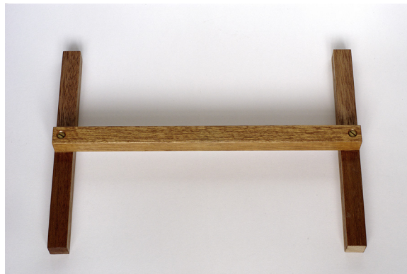
Figure 3.50 This easily-made mahl stick prevents accidental contact with the PCB.
