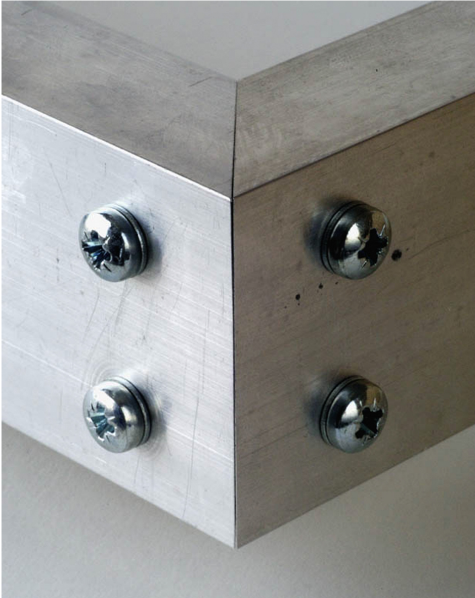
Figure 2.47 Mitred corner joints avoid wasting internal chassis space.
