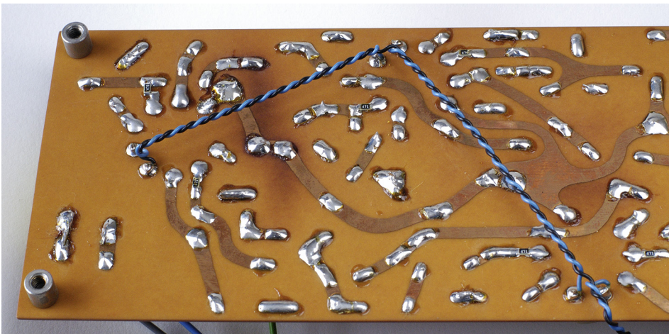
Figure 3.47 Heater wiring on a PCB is best achieved with a twisted pair.
