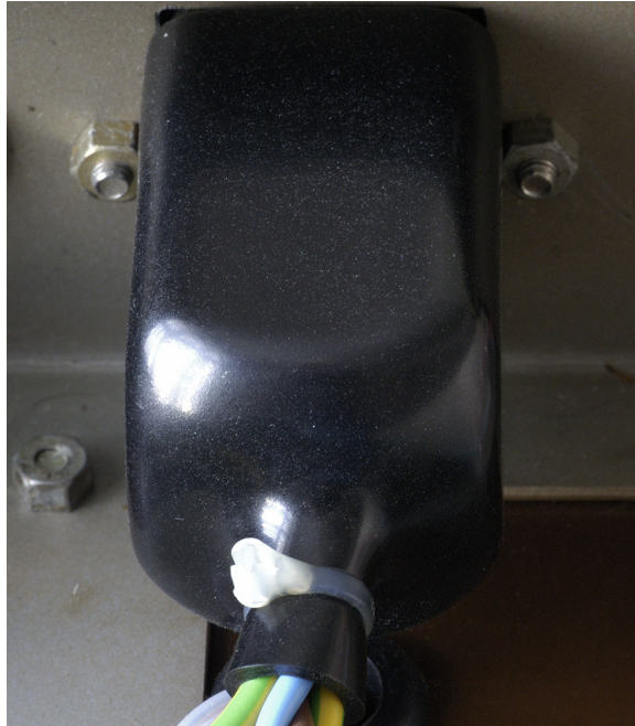
Figure 3.30 IEC input connector sleeved with insulating boot.
