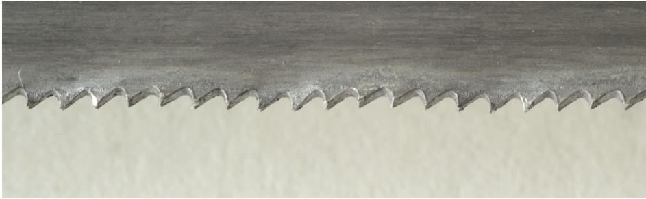
Figure 2.27 Detail of standard hacksaw blade showing cutting direction (blade cuts when moving from right to left).
