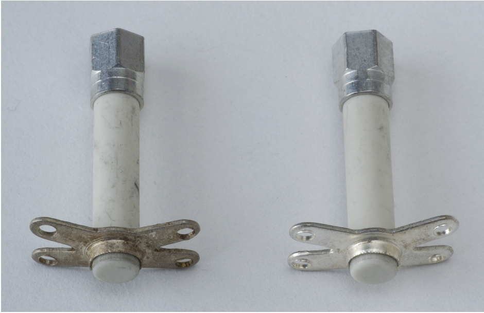
Figure 3.58 Silver-plated tags before and after dipping in “Silver Dip”.
