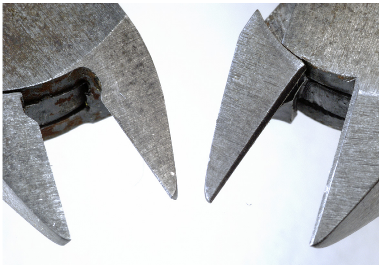
Figure 3.7 Note the difference between flush and semi-flush cutting edges.
