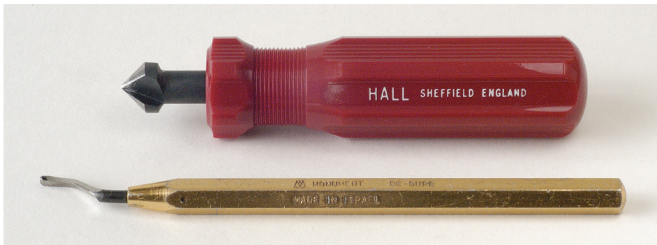
Figure 2.17 “Wiggly” deburring tool (lower) and rose deburring tool (upper).
