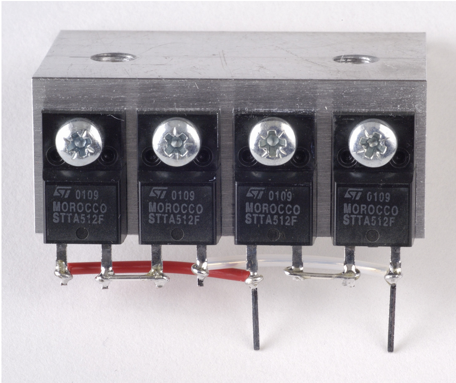
Figure 3.36 Insulated diodes make bridge rectifier construction easier.
